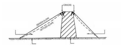
**A)** The fact that the freeboard provided to shield the structure against overtopping by waves was insufficient.
