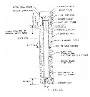
**A)** The presence of relief wells in a dam or levee tends to increase the total quantity of seepage beneath the structure.
