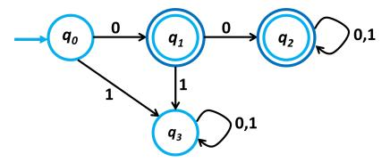
By taking the string 000, the automaton will respond with the state transition sequence  $q_0 \rightarrow q_1 \rightarrow q_2 \rightarrow q_2$ ; since  $q_2$  is a viable final state, we conclude that the machine can accept the string 000. Upon taking the string 010, the automaton will exhibit the state transition sequence  $q_0 \rightarrow q_1 \rightarrow q_3 \rightarrow$  $q_3$ ; noting that  $q_3$  is *not* a viable final state, we surmise that the machine will reject the string 010.
