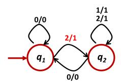
Upon receiving a 1, the machine remains at state  $q_2$  and outputs a 1, as highlighted below.
