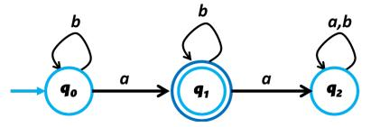
**Problem 2.2:** The DFA below describes an accepter that takes inputs containing at least one a. Starting at  $q_0$ , an input a will cause the accepter to migrate from  $q_0$  to  $q_1$ , which is the final state. Once at  $q_1$ , any input, be it a or b, will not transition back to  $q_0$ ; that is,  $q_1$  functions as a trap state.
