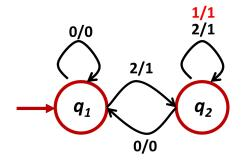
Upon receiving a 0, the machine transitions to state  $q_2$  and outputs a 0, as highlighted below.
