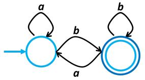
It remains to sketch the state diagram of the machine that accepts the intersection of  $L_1$  and  $L_2$ , as shown.
