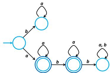
**Problem 2.6:** Consider the language  $L = \{w \mid w \text{ has an odd number of } a's and ends with a b\}$ . The language L is the intersection of two simpler languages  $L_1$  and  $L_2$  such that  $L_1 = \{w \mid w \text{ has an odd number of } a's\}$  and  $L_2 = \{w \mid w \text{ ends with a } b\}$ . The state diagram of the DFA that accepts  $L_1$  is sketched below.
