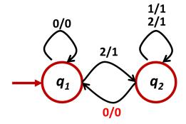
Upon receiving a 0, the machine remains at state  $q_1$  and outputs a 0, as highlighted on the next page.
