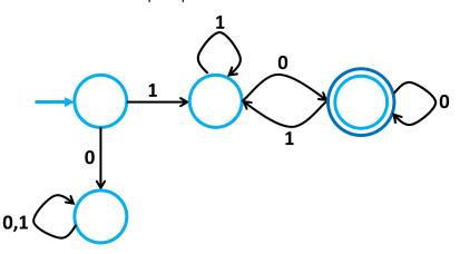
**Problem 3.2:** The state diagram in question is shown on the next page. Beginning at the initial state, the automaton transitions along three vertices, all of which are not acceptable final states because the length of *w* must be at least 3. At the third such node, taking a 1 will displace the system to a trap state, because the third symbol of *w* should be a 0; if the system takes a zero at the third node, an acceptable final state will be reached.
