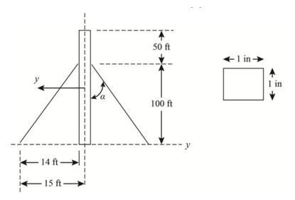
The length  $l_c$  of the cables is calculated as
