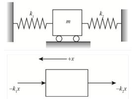
Applying Newton's second law of motion to the block, we have
