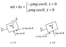
Accordingly, the friction force has the form  $F_f = \mu mg \cos \theta$  and the decrease in amplitude per cycle follows as
