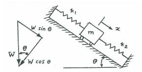
Let x be measured from the position of mass at which the springs are unstretched, and  $\delta$  be the elongation of the springs. The system's equation of motion is
