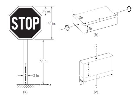
A) The mode of vibration will be transverse vibration about the *xz* plane.
