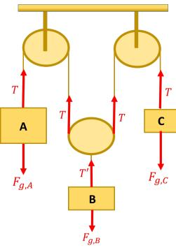
Applying Newton's second law to block A brings to  $T - m_A g = m_A a_A \rightarrow T - 3 \times 9.8 = 3 \times a_A$
