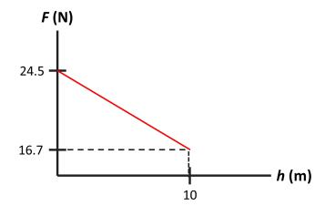
The work done by the operator is given by the area under the graph,
