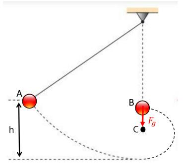
At this point, the tension in the string approaches zero and the sole centripetal force acting on the mass is the weight  $F_g$ ; in mathematical terms,
