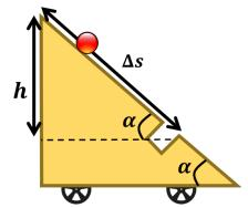
As the ball travels downhill, it covers a distance  $\Delta s = h/\sin \alpha$ . From kinematics, we can determine the time required to cover this distance,
