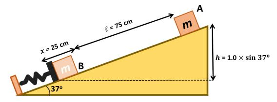
The variation in mechanical energy equals the work of the nonconservative forces. In the case at hand, the only NCF that does work is the friction force f; in mathematical terms,
