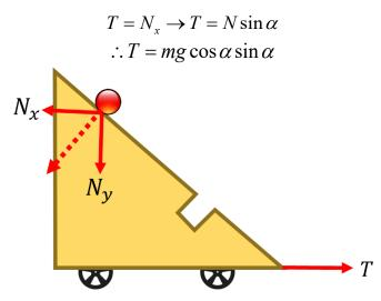
Tension *T* is an external force and adds a linear momentum  $T\Delta t$  to the system. In the period of observation, the system begins with a linear momentum  $Q_i = 0$  and ends with a linear momentum  $Q_f = (M + m)V$ , where *V* is the velocity we aim to determine. Thus,
