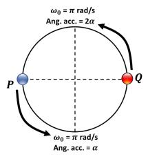
Before anything else, we must determine angular acceleration  $\alpha$ . To do so, we write an equation for the relative motion of the two bodies, noting that, in relative terms, P is  $\pi$  rad ahead of Q until the two bodies collide. Thus,
