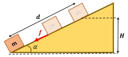
The work of nonconservative forces accounts for the variation in mechanical energy. As shown above, the only NCF that does work in the block's ascending trajectory is the friction force f. As the block travels upward, we have
