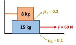
**4.** A 8-kg block is placed on top of a 15-kg block. A horizontal force *F* of 60-N intensity is applied to the lower block, and the upper block is tied to the wall. The coefficient of kinetic friction between the upper block and the lower block is  $\mu_1 = 0.2$ , while the coefficient of kinetic friction between the lower block and the ground is  $\mu_2 = 0.1$ , as shown. If the upper block does not slide relatively to the lower block, the tension in the string is, most nearly:
