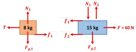
In the upper block, normal force  $N_1$  equals the block's weight  $F_{g,1}$ ; that is,
