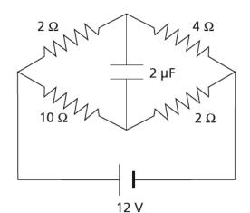
**25.** In the circuit shown, the capacitor has already been fully charged. What is the charge in the  $2-\mu F$  capacitor?
