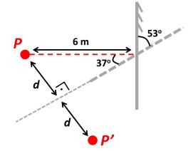
Noting that  $d = 6 \sin 37^\circ = 3.61$  m, the distance from *P* to the new image is calculated to be
