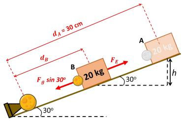
The work done by the electrical force should account for the variation in mechanical energy between points A, at the start of the sliding trajectory, and B, in which the block has reached maximum speed. We shall use point B as a datum for zero gravitational potential energy. In mathematical terms,
