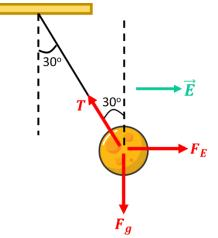
Tension T in the string can be found by adding forces in the vertical,
