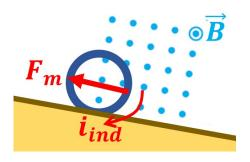
Also in furtherance of the  $t_2 > t_1$  conclusion is the fact that, as the ring traverses the magnetic field in situation 2, the induced current that flows in the ring causes it to heat up by Joule effect. This thermal energy comes at the expense of kinetic energy and ultimately contributes to the deceleration of the ring.
