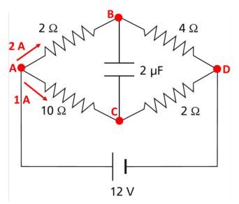
Equipped with the current values, we can establish the potential difference  $U_{BC}$  across the capacitor. First, we apply Ohm's law to segment AB,
