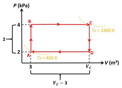
Now, determining the work done in cycle *ABCD* becomes merely a matter of establishing the area of rectangle *ABCD*, namely
