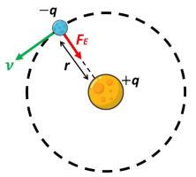
The energy to be added to the system equals  $\Delta E = E_1 - E_0$ , where  $E_0$  is the energy of the system when the orbit has a radius of 0.5 Å and  $E_1$  is the energy of the system when the orbit has a radius of 1 Å. The energy in either state is given by the sum of an electric potential energy component, U, and a kinetic energy component, KE; mathematically,
