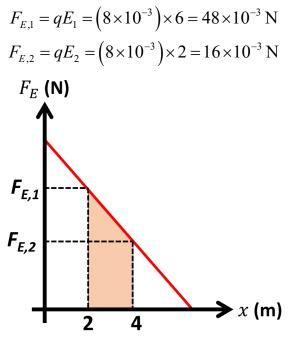
The area under a graph of force versus distance yields work; in the case at hand,
