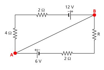
**22.** The circuit is powered by two batteries. What is the value of the current in wire *AB* if resistance *R* equals  $10 \Omega$ ?
