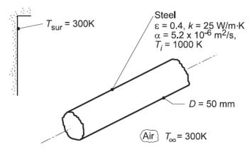
The film temperature is  $T_f = (T_i + T_\infty)/2 = (1000+300)/2 = 650$  K, and consequently  $\beta = 1/T_f = 1/650 = 0.00154$  K<sup>-1</sup>. The Rayleigh number is
