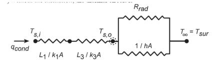
The outer surface temperature  $T_{s,o}$ , which is our main unknown, is highlighted. Performing an energy balance at the outer surface, we write
