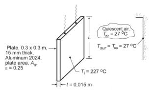
From an energy balance on the plate with free convection and radiation exchange, we obtain
