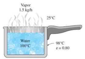
**A)**  $\dot{q}_{conv} = 23.1$  W and  $\dot{q}_{rad} = 28.6$  W **B)**  $\dot{q}_{conv} = 23.1$  W and  $\dot{q}_{rad} = 47.3$  W **C)**  $\dot{q}_{conv} = 46.2$  W and  $\dot{q}_{rad} = 28.6$  W **D)**  $\dot{q}_{conv} = 46.2$  W and  $\dot{q}_{rad} = 47.3$  W
