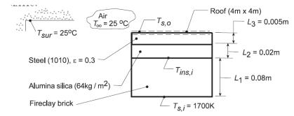
Without the insulation, the thermal circuit is as shown.
