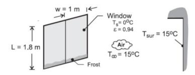
For these winter conditions, a frost line could appear and it would be at the bottom of the window. The boundary layer is thinnest at the top of the window, and hence the heat flux from the warmer room is greater than compared to that bottom portion of the window, where the boundary layer is thicker. Also, the air in the room may be stratified and cooler near the floor compared to near the ceiling.
