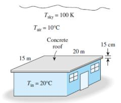
**A)** *q̇* = 35,700 W **B**) *q̇* = 43,900 W **C**) *q̇* = 51,500 W **D**) *q̇* = 60,100 W
