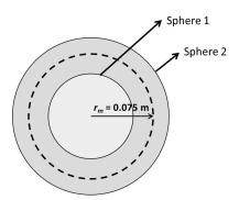
The conduction heat rate into the dashed control surface must equal the conduction heat rate out of the control surface. Thus, we can propose the equality
