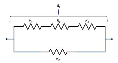
The overall thermal resistance  $R_{total}$  is then
