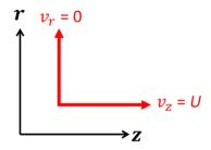
For a uniform stream moving from left to right,  $v_r = 0$  and  $v_z = U$ . Integrating  $v_z$  brings to
