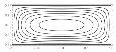
We could just as well plot contours for a section with aspect ratio equal to, say, 0.8, and 25 terms in the summation (although using only about 5 or 6 terms is quite adequate for most purposes):
