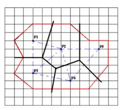
We then take the product of the area of each polygon and the precipitation of the basin located within it, and finally obtain the average precipitation by dividing the sum of  $A \times P$  products by the area of the basin; that is,  $P_{Avg} = \Sigma (A \times P)/A_{Basin}$ . The calculations are summarized in the following table.
