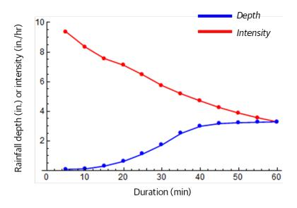
It is noticed that the mass curve sharply increases before the peak and then becomes flatter as time increases, while the *P-I* curve falls continuously with time. The two curves meet at the end of the storm time, on a point that is numerically equal to the largest cumulative depth (= 3.29 in.).
