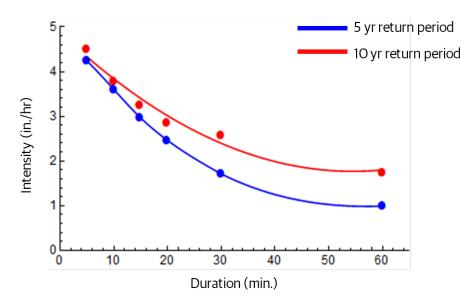
Finally, the IDF curves are obtained by plotting intensity, in in./hr, versus duration, in min.
