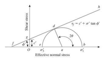
The failure envelope is *fgh*, and follows the equation  $\tau_f = c' + \sigma' \tan \phi$ . The radial line *ab* defines the major principal plane, and the radial line *ad* defines the failure plane. It can be shown that the angle  $b\hat{a}d = 2\theta = 90 + \phi'$  or, equivalently,  $\theta = 45^\circ + \phi'/2$ . (We take advantage of this result in some of the following
