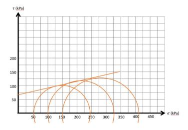
We thus obtain shear strength parameters c' = 70 kPa and  $\phi'$  = 15°.
