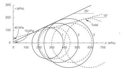
The effective failure parameters are found to be c' = 10 kPa and  $\phi' = 25^{\circ}$ .
