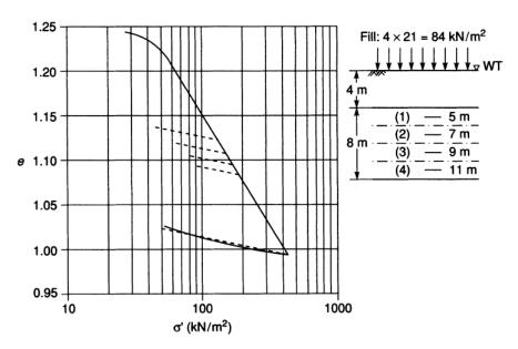
Then, the following table is prepared. In the second column the initial stress  $\sigma'_o$  is the product  $(4 + 1) \times (19.0 - 9.8) = 46 \text{ kN/m}^2$ , where the first factor is the depth from the surface to the middle of the first layer and the second is the submerged unit weight of either soil. The third column, in turn, is the sum of the aforementioned 46 kPa and the stress due to the overlying sand fill,  $4 \times 21 = 84$  kPa, totaling  $\sigma'_1 = 46 + 84 = 130$  kPa.
