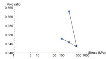
**Part B:** The compression index is the average slope of the normal consolidation line in a plot of void ratio versus the logarithm of stress; mathematically,
