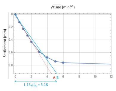
Finally, the intercept of the blue line with the settlement-time<sup>1/2</sup> curve is to be taken as the time required for 90% consolidation,  $t_{90}$ . Projecting the intercept onto the abscissa yields  $\sqrt{t_{90}}$ .
