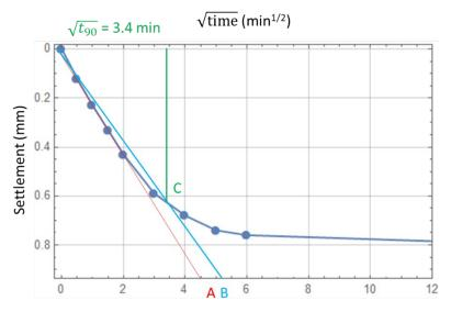
The green line intercepts the horizontal axis at  $\sqrt{t_{90}} \approx 3.4$  min., which corresponds to a time of 90% consolidation  $t_{90} = 11.56$  min. We are then ready to substitute the available data in the expression for the time factor  $T_{\nu}$ , which can be easily solved for the coefficient of consolidation,
