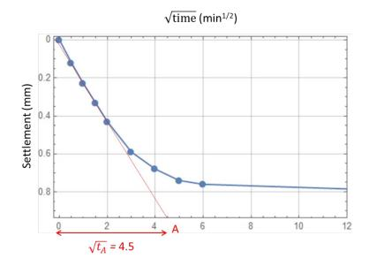
It is found that  $\sqrt{t_A} = 4.5 \text{ min}^{1/2}$ . The next step is to draw a second line, this time going from the origin to the abscissa corresponding to  $1.15\sqrt{t_A} = 1.15 \times 4.5 = 5.18 \text{ min}^{1/2}$ ; the line in question is shown in blue below.
