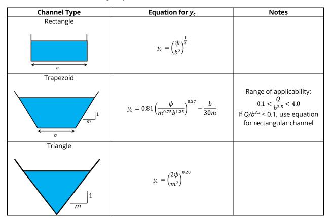
Using Straub's formulas, find the critical depth for a trapezoidal channel with 5 m width and side slope m = 1 carrying a discharge of 8 m<sup>3</sup>/s. Assume  $\alpha = 1.0$ .
