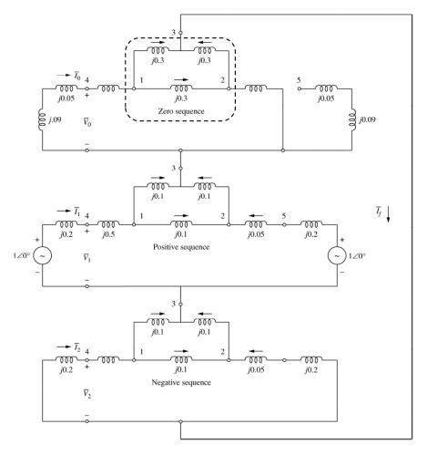
From the solution to Problem 14.1,  $I_f = -j1.8214$  pu. From the circuit above,  $I_1 = I_2 = I_f/2 = -j0.9107$  pu. Transforming the  $\Delta$  of j0.3 in the zero sequence network (highlighted by dashed lines above) into an equivalent Y of j0.1 and using current division,
