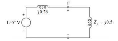
The fault current for a balanced three-phase fault is calculated to be
