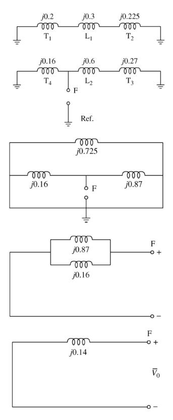
We calculated a final reactance of j 0.14 pu for the positive sequence network. As stated, a j 0.5-pu impedance is added to the network.
