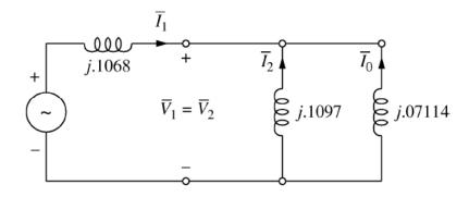
Referring to the diagram above, current  $I_1$  is determined as
