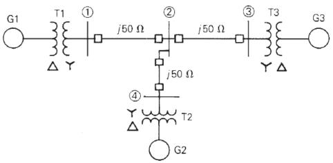
**Problem 12.1:** The inductor connected to generator G3 neutral has a reactance of 0.028  $\Omega$ . Draw the zero-, positive, and negative-sequence reactance diagrams using a 1000-MVA, 20-kV base in the zone of generator G3. Neglect  $\Delta$ -Y transformer phase shifts.
