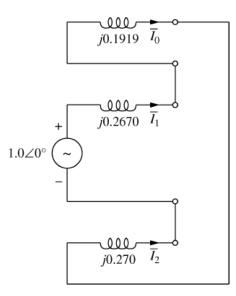
The sequence current through each impedance is the same, and can be calculated as
