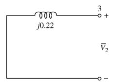
The zero-sequence network is shown below considering the transformer winding connections (as before, I'd suggest converting the  $\Delta$  to a Y with four decimal places only, instead of the six used in the illustration).
