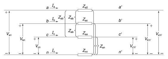
**Problem 3.2:** Show that the sequence components of the voltage drops between the ends of the line section can be written as  $V_{aa'0} = Z_0I_{a0}$ ,  $V_{aa'1} = Z_1I_{a1}$ , and  $V_{aa'2} = Z_2I_{a2}$ , where
