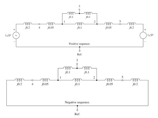
Using delta-wye transformation and series-parallel combinations, Thévenin equivalents looking into bus 3 are shown below.
