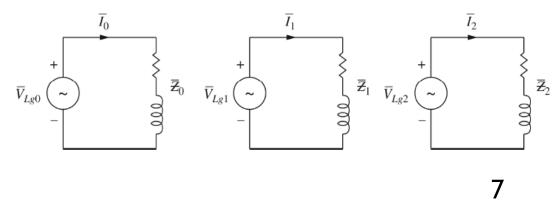
Given  $V_{L,g0} = 5.04 \angle -57.6^\circ$ ,  $V_{L,g1} = 273 \angle 6.59^\circ$ , and  $V_{L,g2} = 27.8 \angle -76.0^\circ$ , we compute the sequence components of the line currents as follows,
