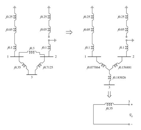
For a single line-to-ground fault through a fault impedance  $Z_F = 0.1$  pu, we draw up the following interconnections.
