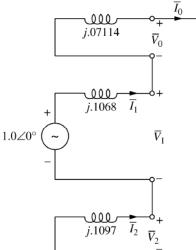
The pertaining reactances have been determined above. The zero-, positive-, and negative-sequence current components are given by
