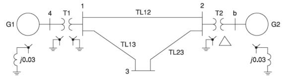
**Problem 14.1:** Using a 100-MVA, 230-kV base for the transmission lines, draw the per-unit sequence networks and reduce them to their Thévenin equivalents, "looking in" at bus 3. Neglect  $\Delta$ -Y phase shifts. Compute the fault currents for a bolted three-phase fault at bus 3.
