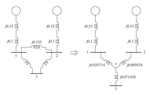
Converting the  $\Delta$  formed by buses 1, 2 and 3 to an equivalent Y, we have (my calculations use less decimal places than the illustration above)
