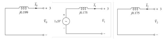
A bolted three-phase fault occurs at bus 3.
