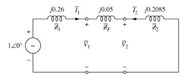
Current components  $I_{\rm 1}$  and  $I_{\rm 2}$  flow in opposite directions and have intensity given by
