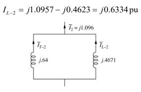
We proceed to determine the contributions to fault current from transformer,
