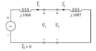
Current components  $I_{\rm 1}$  and  $I_{\rm 2}$  flow in opposite directions and are given by
