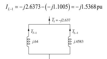
For negative sequence, recalling that  $I_2 = j1.0957$  pu, the contributions from transformer and line are
