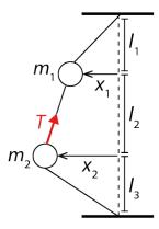
The horizontal (along the  $x_1$ -direction) components of tension in the string lying above and below  $m_1$  are  $-x_1T/l_1$  and  $-(x_1 + x_2)T/l_2$ , respectively. Thus, we can write Newton's second law for mass  $m_1$  as
