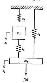
**A)** One of the natural frequencies is  $\omega = 0.60\omega_n$ . **B)** One of the natural frequencies is  $\omega = 2.36\omega_n$ . **C)** One of the mode shapes is  $X_2 = 1.28X_1$ . **D)** One of the mode shapes is  $X_2 = -0.785X_1$ .
