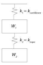
The stiffness of the cantilever beam,  $k_1 = k_{cantilever}$ , is given by
