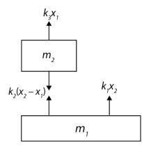
Let the free responses be described by  $x_1 = X_1 e^{st}$  and  $x_2 = X_2 e^{st}$ . Applying Newton's second law to mass  $m_1$ , we can write
